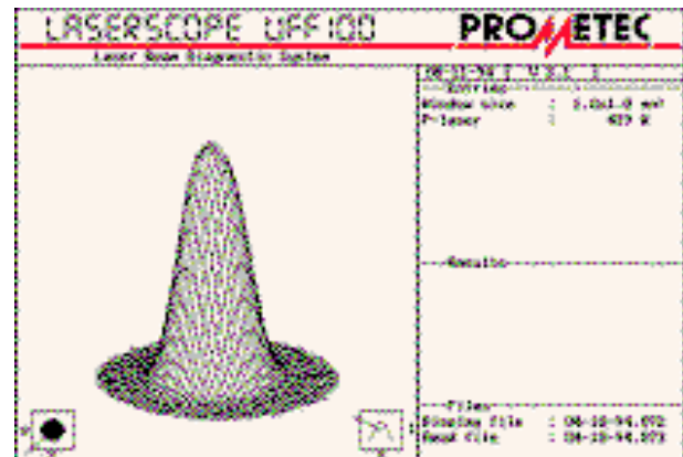
(c) Focused beam exiting a gradient-index fiber.
