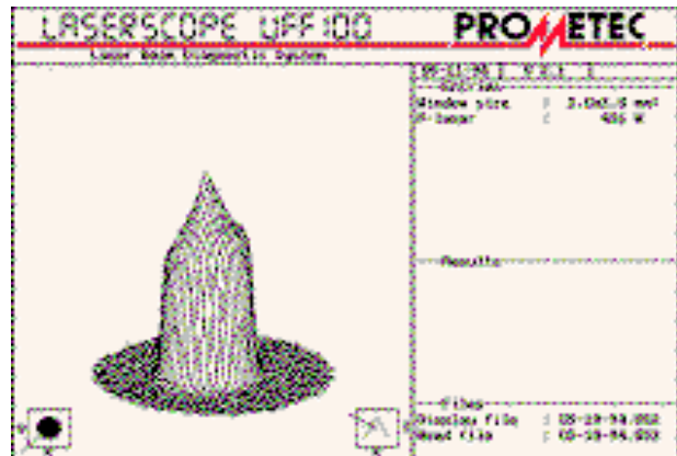
(b) Focused beam exiting a step-index fiber.
